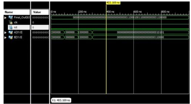
Fig. 5.3: The output waveform of a RoBA Multiplier.
