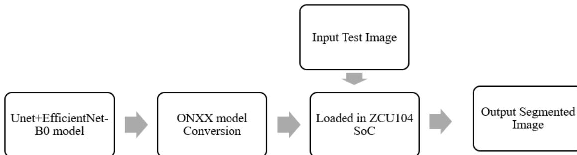
Fig. 2: Block Diagram of SoC Implementation
