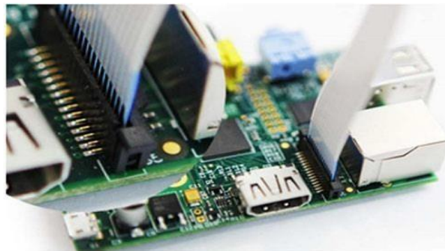
Fig. 4: Camera serial interface of Pi
